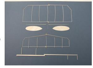
in position, holding them in place with soft balsa "clamps", don't pin the spars directly. You should pre glue all joints. I attach the ribs first at the leading edge, then cut to length using a NEW piece of razor blade and glue to the trailing edge.
